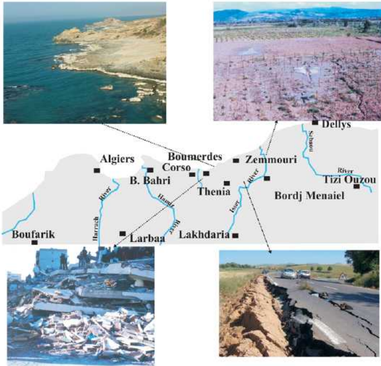
Fig. 2. Surface effects and damage in the epicentral area are shown. No surface faulting was visible inland. Photos: Upper left, coastal uplift (average 0.5 m) marked by the intertidal zone (white band); upper right, liquefaction features (sand blows); lower left, "pancake" building collapse; lower right, secondary surface cracks.
